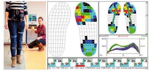
Figure 2. a. Pedar-X system for measuring in-shoe plantar pressure during walking with and without foot orthoses developed according to the protocol b. Feedback generated by the system, identifying regions of high plantar pressure.
